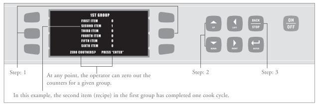
FIGURE 22: Checking the Recipe Counter
